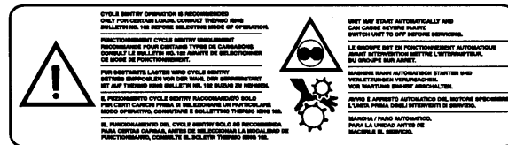
Figure 8: Automatic Start Caution (Locations vary depending on model. Decals are located near areas that contain moving parts which can cause severe injuries if hands or clothing become tangled when the unit automatically starts.)
