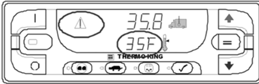
Figure 26: Alarm Icon and Setpoint
