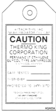
Figure 5: Antifreeze Caution (Attached near radiator fill cap.)
